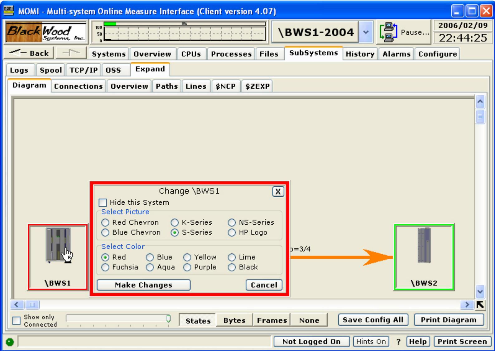
Placing the mouse over a connection between two Systems and clicking will bring up a detailed diagram of the connections, states, frame rate and byte rate between the two nodes. Frame rate and byte rate (if available) are also displayed for each line and a total for the path.
